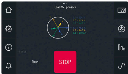
In-line/load phasor diagram
