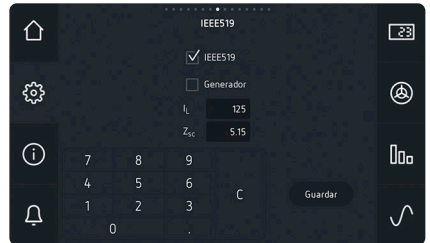
Filters harmonics as per IEEE 519
